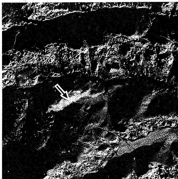
Figure 8 - KVR-1000 orthoimage showing badland areas east of Alianello. Relief changes are clearly revealed.
