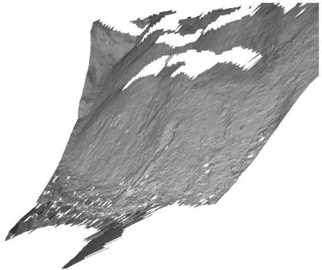
Figure 4. Digital elevation model (rendered) after geocoding. White areas within the DEM could not be measured due to occlusions.
