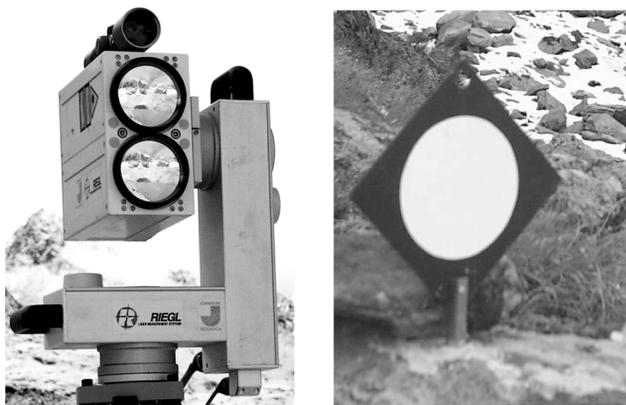
Figure 1. Left: Laser scanner LPM-2k by Riegl Laser Measurement Systems. Right: Reflective reference target used for sensor orientation.
