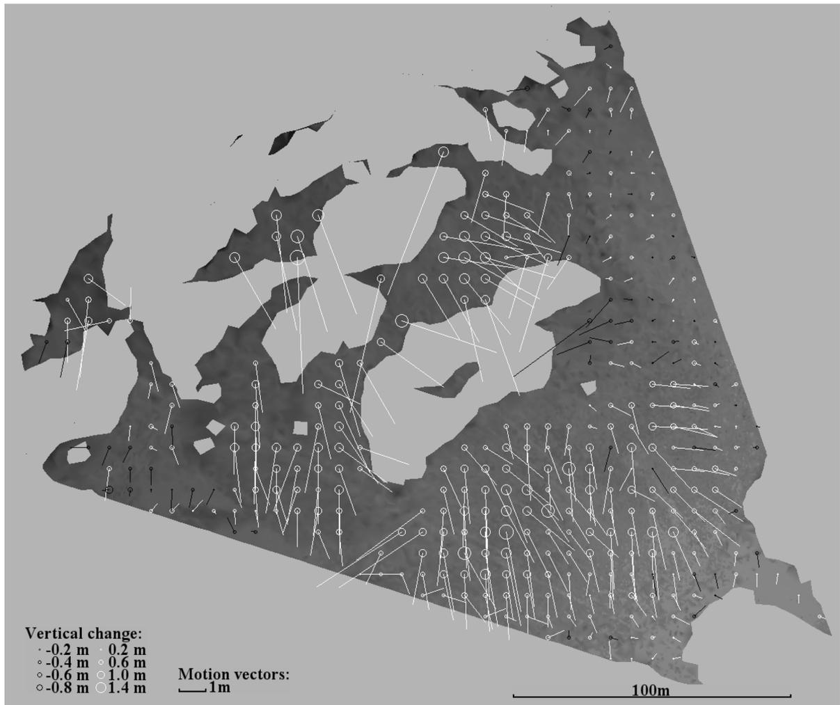
Figure 7. Results of surface structure matching: Change between August 2000 and August 2001. Circles describe vertical changes, the vector field displays the horizontal movement.
