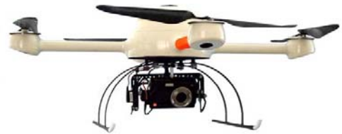
Figure 1: Micro-drone md4-200 with attached PENTAX Optio A40.
