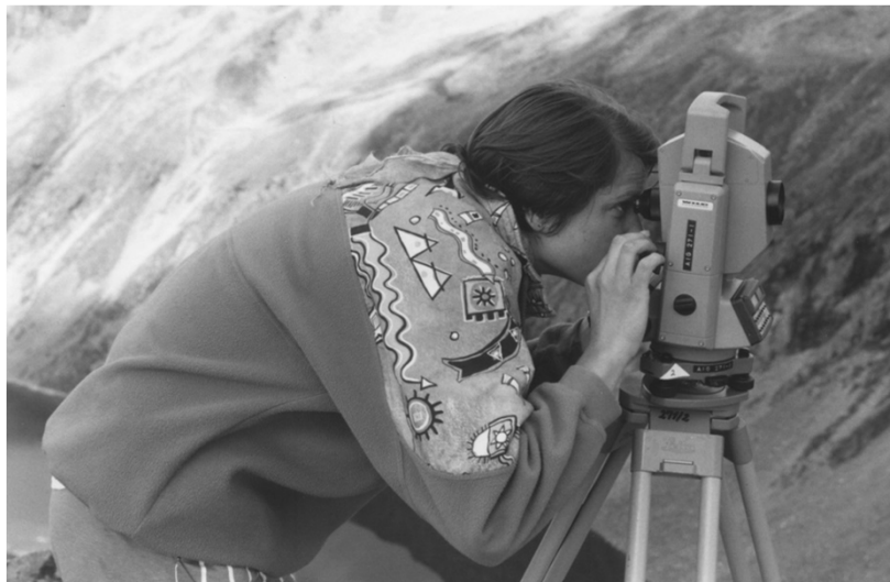
Polar method surveying from point S4
