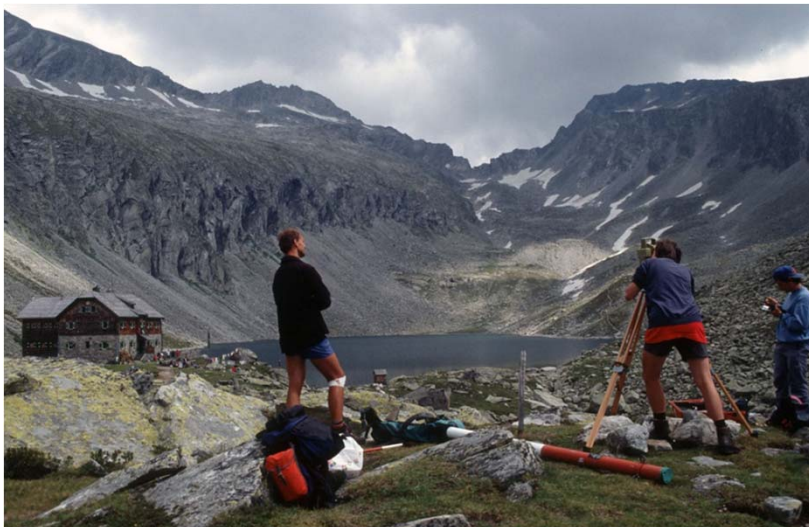
Geodetic survey at the triangulation point AVS
