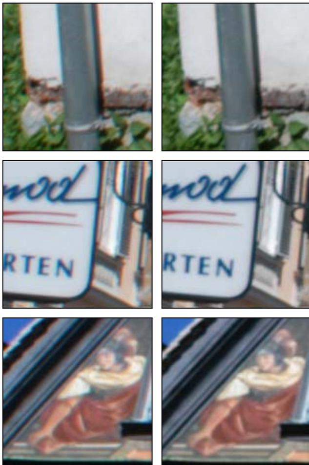
Figure 12. Examples for the elimination of color fringes in digital photographs. The photographs were taken with a Nikon D100 digital SLR camera using a 20 mm lens. The image chips shown (window size  $150 \times 150$ ) were cropped from areas near the image corners. The left column shows the original image data, whereas the right one is corrected for. The last example was taken from the photograph (Figure 13) shown below.
