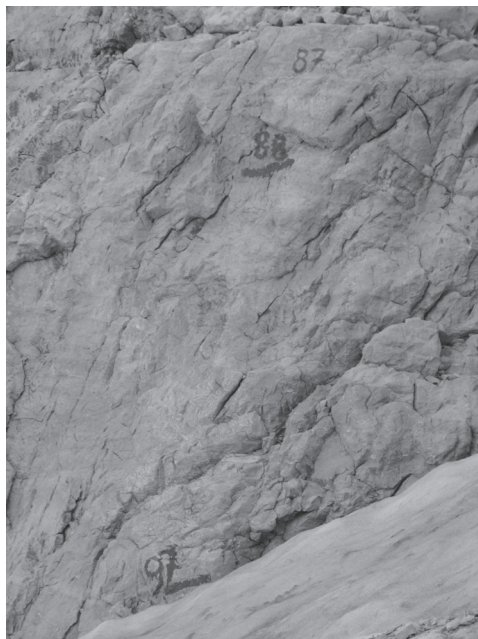
Figure 3: Ground markings (years) to help measure the vertical retreat of the Triglav Glacier with a tape measure (photo: Matija Zorn).
