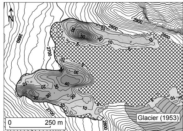
Figure 8. Mean annual horizontal creep velocity ( $\text{cm a}^{-1}$ ) at Inneres Hochebenkar rock glacier for the time period 1953-1969
