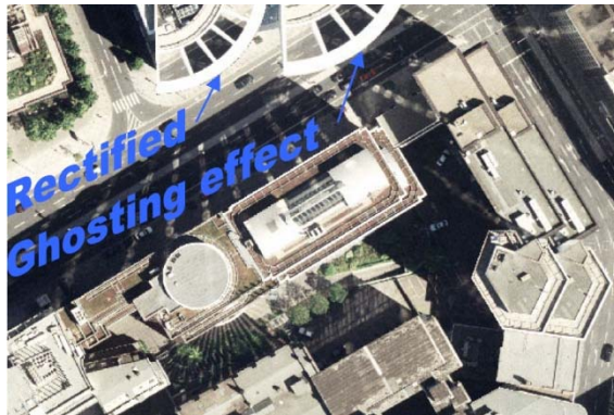
Ghosting effect due to the use of a DSM in a city without detection of occluded areas, even if the building is correctly rectified.
