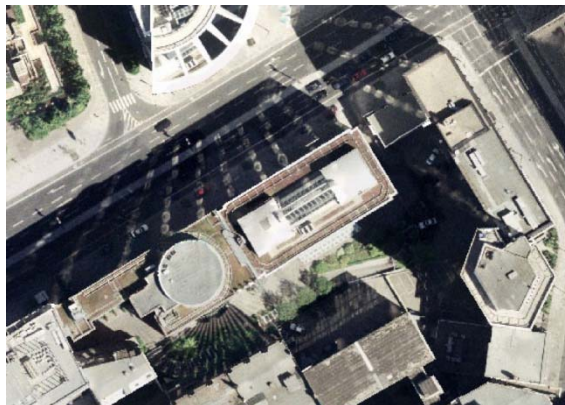
True orthophoto. Occlusions automatically replaced by using several overlapping orthophotos.
